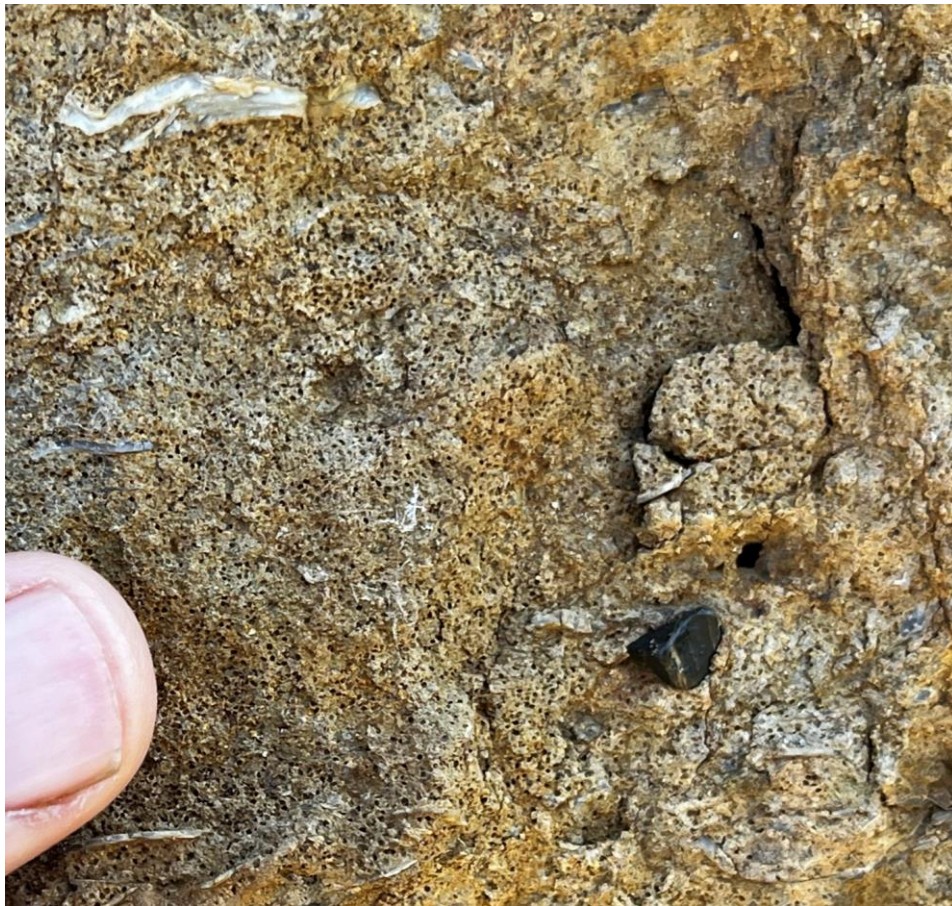
Figure 31 Oolitic shelly ironstone with a calcareous matrix and common shell fragments and scattered lydite pebbles.
