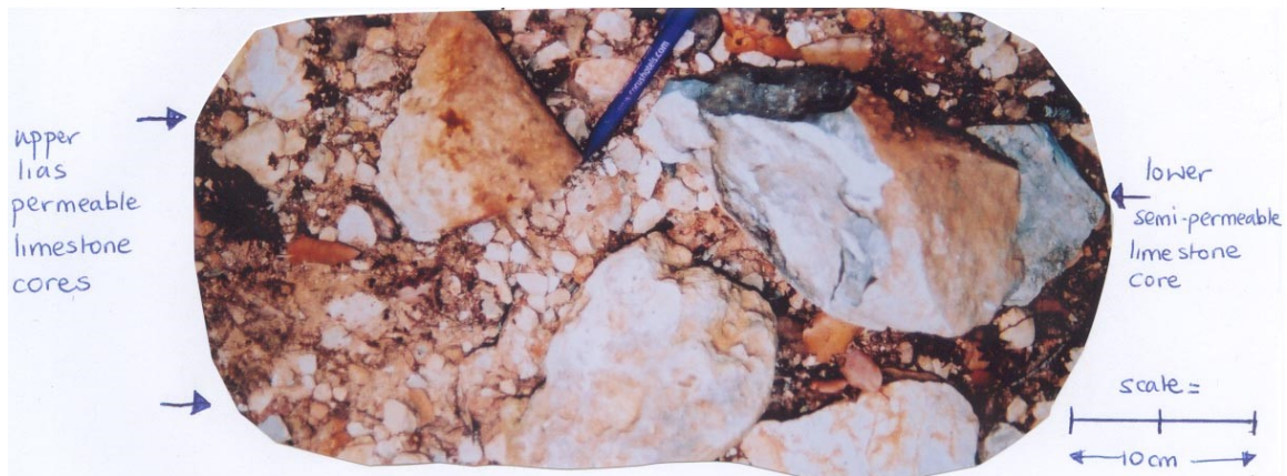
Figure 8. Core samples from Lias limestone and Lower Rhaetic limestone.
